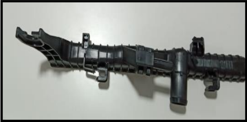
Inlet / Outlet Tank for MATS
